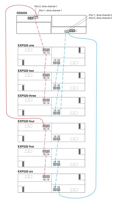
Figure 50. One DS5020 and a maximum of six EXP520 storage expansion enclosures behind a pair of DS5020 drive ports
